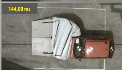
Vehicle still decelerating, whilst keeping direction. It will not be redirected to the driving lane or other obstacles
