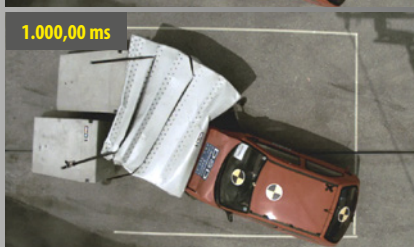
Vehicle stopped moving, driver takes no injury. The F1-80 starts to unfold, soon ready to take the next impact ...
