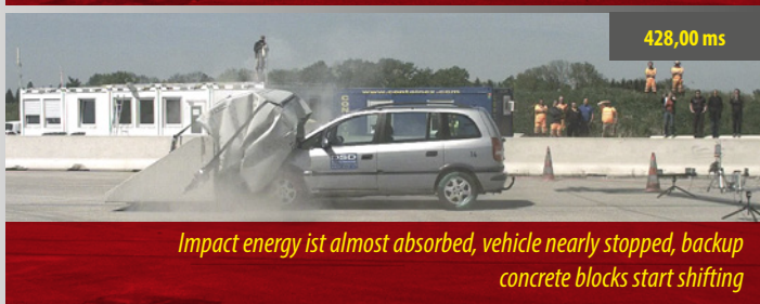
Still slightly decelerating the vehicle, the Road Airbag is compressed to its maximum
