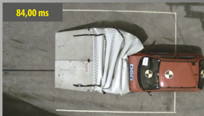
Deceleration of the vehicle in progress, whilst the air valves do their work and transform the impact energy into airflow
