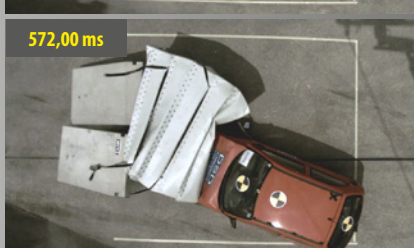
Impact energy almost absorbed, vehicle speed and sideways shifting almost stopped, backup concrete blocks start shifting
