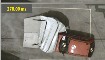
Still slightly decelerating the vehicle, the Road Airbag is compressed to its maximum. Vehicle starts shifting sideways slightly
