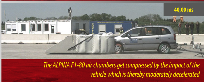
First contact, vehicle hits the front of the impact absorber
