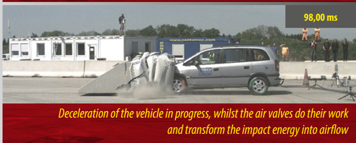
The ALPINA F1-80 air chambers get compressed by the impact of the vehicle which is thereby moderately decelerated
