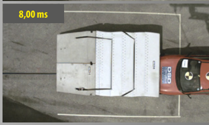
First contact, vehicle hits the front of the impact absorber, but offset from the center
