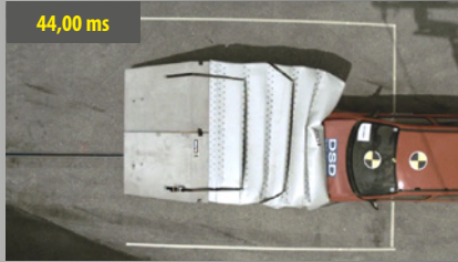
The ALPINA F1-80 air chambers get compressed by the impact of the vehicle which is thereby moderately decelerated
